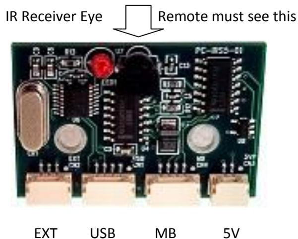
From the back of the IRS5, starting on the right, the connectors are:
